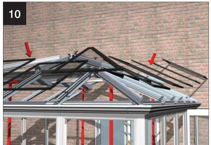
10 Glaze the lower pagoda roof fully.
