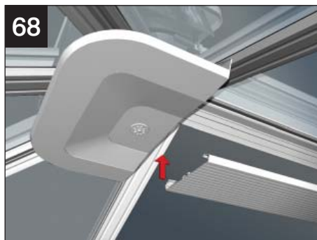
68 Clip the internal ridge cladding onto the underside of the ridge.
