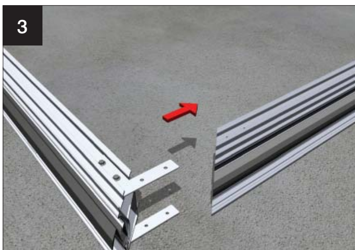
Slide the cleated corners into the adjacent piece of lantern beam
