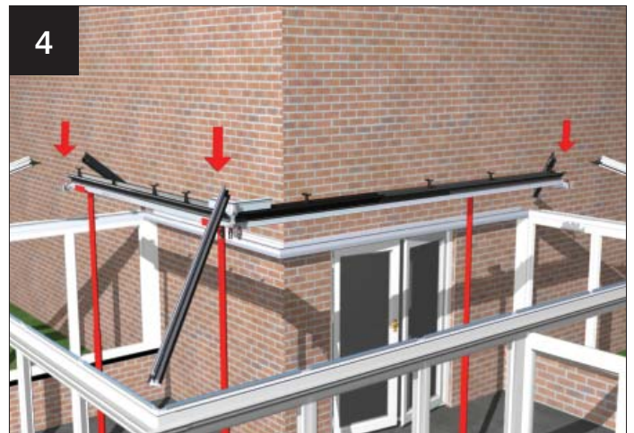
4 Temporary support/prop the 'L' shaped ridge. Offer up the hip bars. Secure using steps 13-18 in the main installation guide. Build remainder of the roof as section 4.
