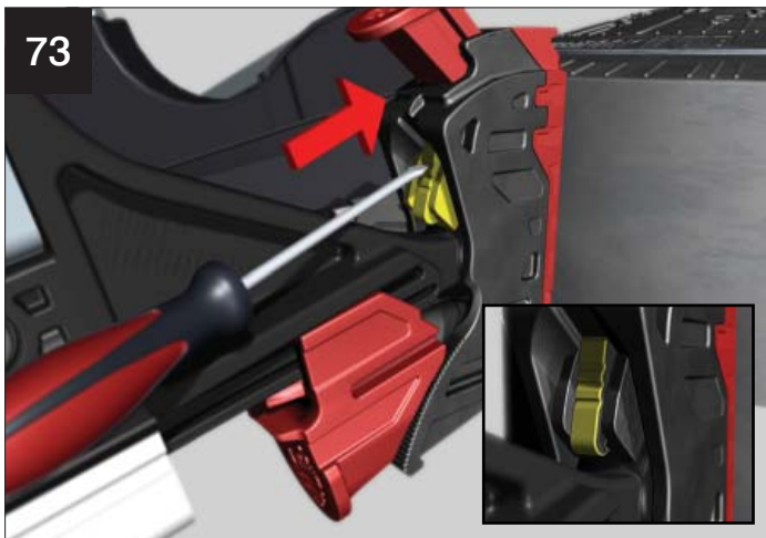
Insert the 5mm wide flat blade screwdriver and gently push against the upper edge of the roller cam (marked yellow).
