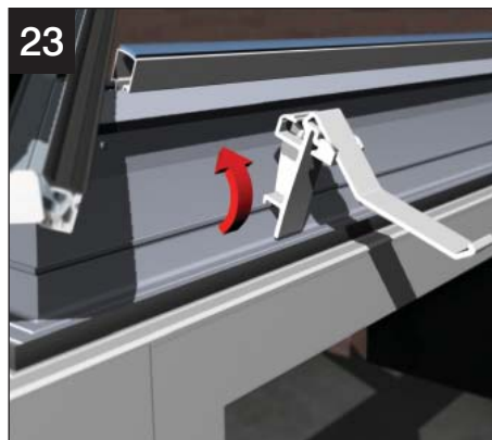
23 Fit all the gutter brackets supplied with the kit at maximum 750mm centres and maximum 200mm from each corner.
