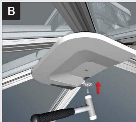
B To fit the internal radius end capping insert the rose fixing button and tap the plastic rivet home to secure the button. On some occasions it may be preferable to test fit the ridge internal cladding prior to fitting the radius end capping.
