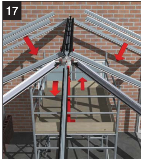
17 Continue to attach all the glazing bars using the location plan provided to check each bars final position with its corresponding label.
