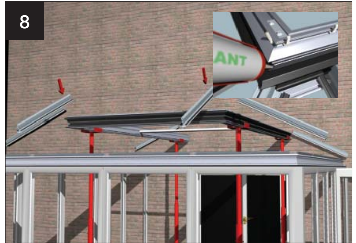
8 Now the Pagoda eaves beam is assembled into a one piece structure, temporarily support it. Attach the glazing bars according to the component location plan. Tighten the bars, at the pagoda beam end first and then at the main eaves beam second. At the corners, seal using a sealant appropriate to the glazing material (shown above).
