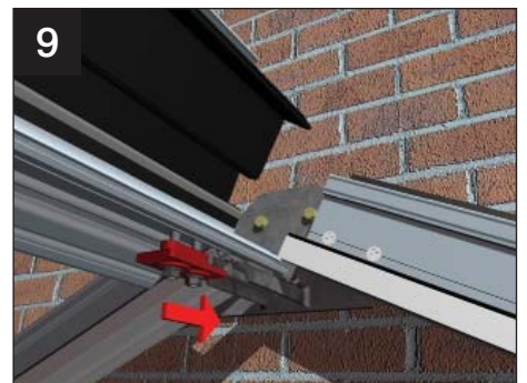
Loosen the "crocodile jaw" bolts on the underside of the main ridge body – ensure it is supported at the front whilst it is gently guided onto the top half of the 'crocodile jaw'.
