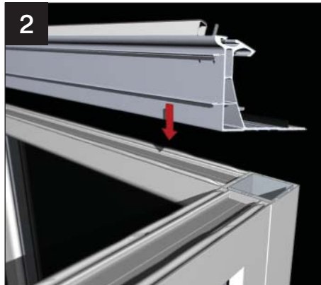
2 Fit the initial piece of eaves beam ensuring that the inside face of the eaves beam is flush with the inside face of the window frame. Please note: Ensure that the under gutter trim is fitted to the eaves beam and all bolts are in situ prior to fixing to the frames.
