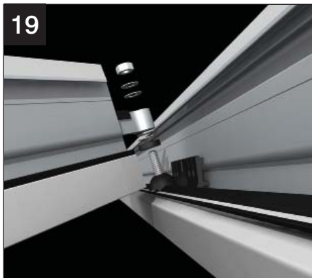
19 Slide back the jack rafter undercladding. Each jack rafter kit is supplied with a number of washers. Trial fit the jack rafter and check that the glazing platforms are level. Adjust if necessary by adding or removing washers between the two part connecting kit, then tighten the nut.
