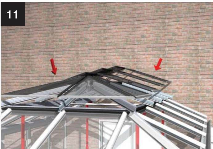
11 Glaze the upper pagoda roof, and complete all external works
