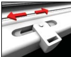
67 Ensure the ventilation button is fixed into the ridge undercladding as shown before you install the cladding.
