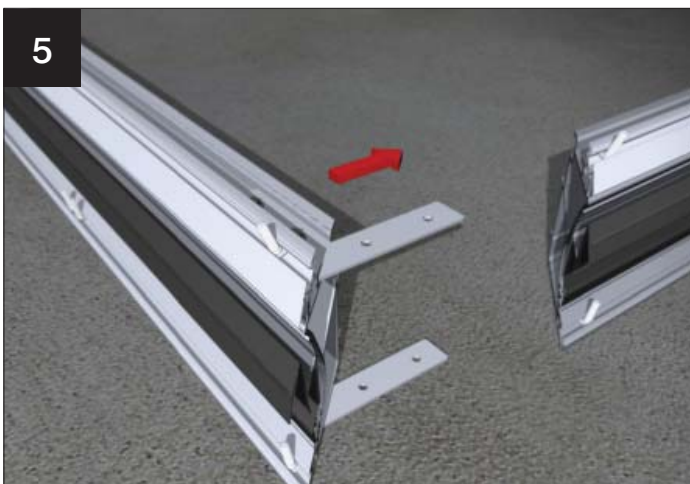
Slide the cleated corners into the adjacent piece of pagoda beam
