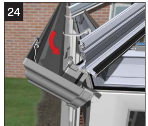
24 Locate the back edge of each section of gutter into the slot in the gutter bracket.
